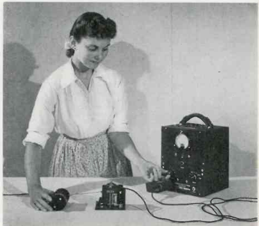
VIBRATION METER, developed by General Electric, shown with aircraft motor, determines vibration velocity and displacement
