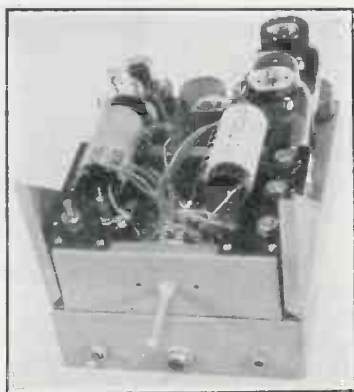
Series 20, 4 channel 1600-6000 K.C., 20 watt transmitter.
