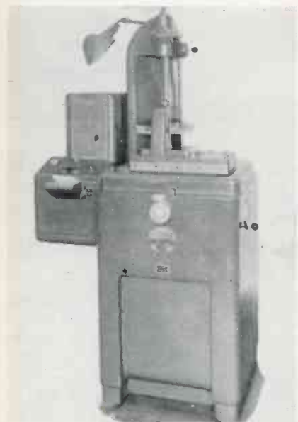
INVOLUTE MEASURING machine equipped with GE chart type electronic recording device manufactured by Fellows Gear Shaper Co.
