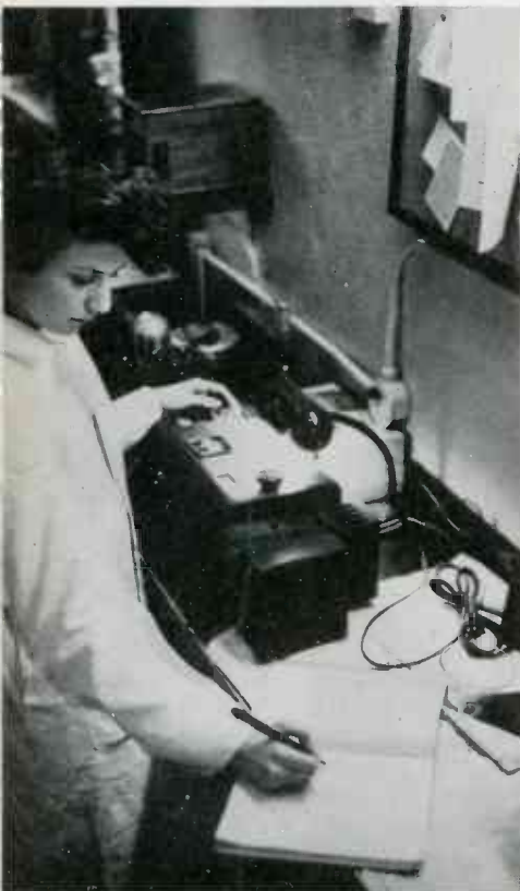
UNABRIDGED SPECTROPHOTOMETER measures light transmission of sample at all wavelengths for most accurate vitamin assays. Diagram of electronic null-point system of Beckman unit below
