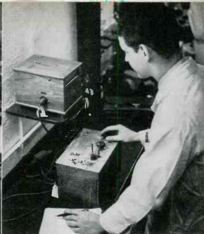
VITAMIN A ANALYSIS at Food Research Labs., Inc., with Rubicon abridged photoelectric spectrophotometer
