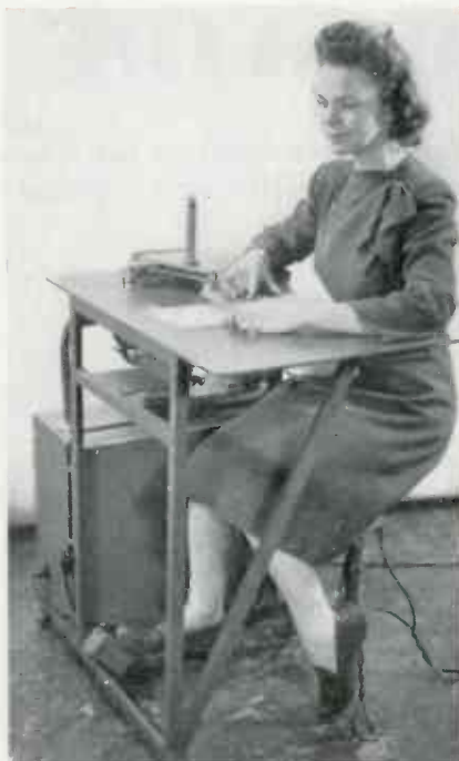
RADIO-FREQUENCY current stitches a thin solid seam that is both air- and water-tight. Developed by RCA for the plastics industry in fabricating thermoplastic materials
