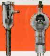
Two electronic tubes, the G-E phanotron and the G-E pliotron, supply the high-frequency waves used in electronic heating.
