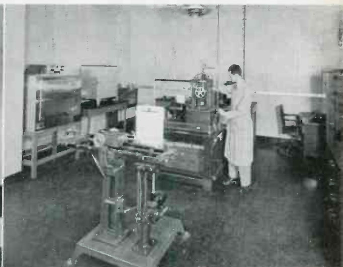
INDIVIDUAL LABORATORIES are completely equipped for the investigation of particular projects. In the one above, an investigation of the physical properties of rubber is under way. Tensile, compression and plasticity tests are conducted here on rubber compounds under controlled temperature and humidity conditions
