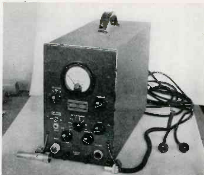
Wide band amplifier (Type 319A) manufactured by RCA adapted to transform the output of a piezo electric gage to operate an oscillograph
