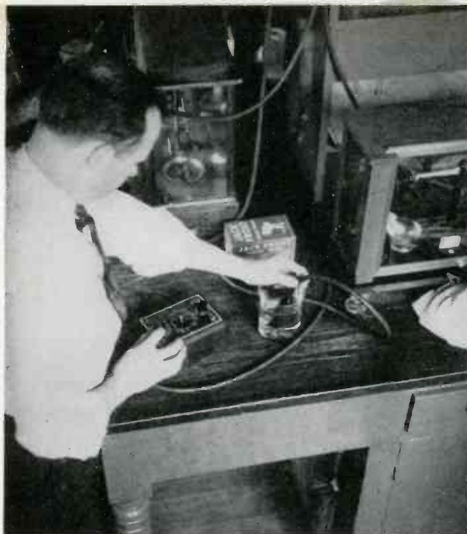
ELECTRON RAY bridge-type conductivity meter checks solutions at National Sugar Refining Co.
